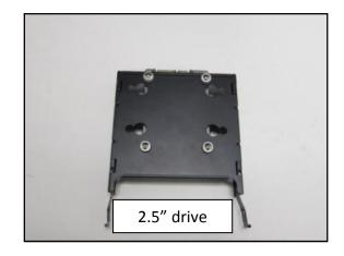
5. Insert the 3.5" / 2.5" drive into the drive cage by pinching the ends of the drive tray and sliding the tray along the rails until the tray locks firmly into position.
